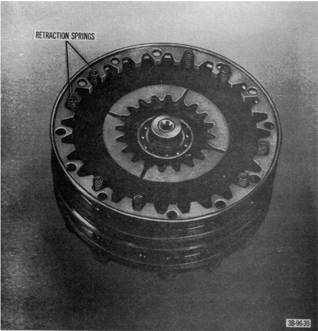
Figure 51. Retraction springs installed in slots of clutch ring.
